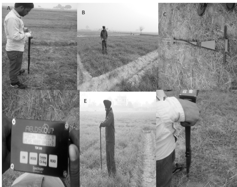
Fig 1. Photographs showing the recording of volumetric moisture content up to 7.5 cm using time domain reflectometer (TDR)
